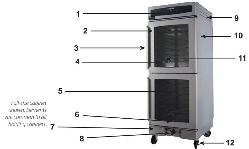
1. **Control Panel** - contains power button and control escutcheon. Allows operator to program food temperature and food texture. Escutcheon is removable for servicing or replacing microprocessor.
